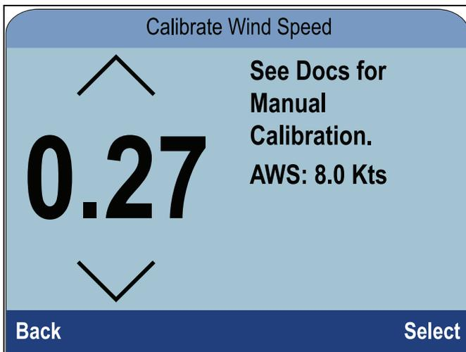
The Calibration Factor default is 1.00 the Calibration Factor can be adjusted from 0.25 to 2.00.
