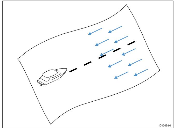
With your vessel sailing directly into the wind the Apparent Wind Angle (AWA) should be 0 degrees.
