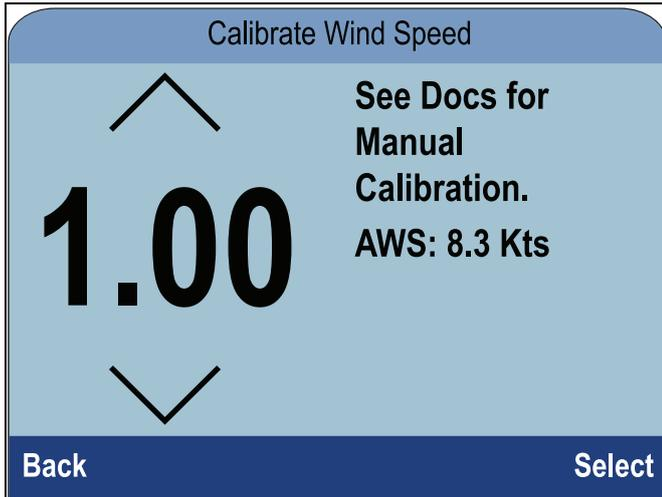
4. Use the **Up** and **Down** buttons to adjust the Calibration Factor until the AWS reading matches your referenced source of AWS.
