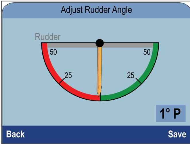
5. Use the **Up** and **Down** buttons to adjust the pointer so that the pointer and the reported Rudder Angles are both zero.
