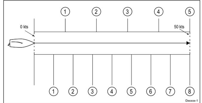
With the Speed Transducer connected to a Speed Pod the 5 calibration points are fixed in sequence at 2, 4, 8, 16 and 32 knots. When adding calibration points during the Speed Run Calibration ensure vessel speed is as close to the fixed calibration point speeds as possible, as the calibration factor applied will be the difference between the actual vessel speed and the fixed calibration point speed.
