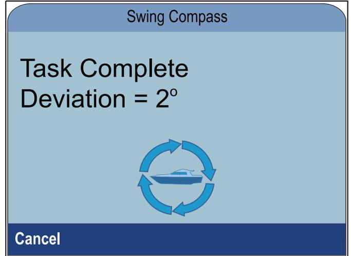
10. If the deviation is greater than 15 degrees you will need to relocate the Compass further away from metal items or items that may cause interference, then repeat the calibration process. If you still find a deviation of more than 15 degrees, contact your Raymarine dealer for advice. If the deviation is within acceptable limits, press **Cancel**.
