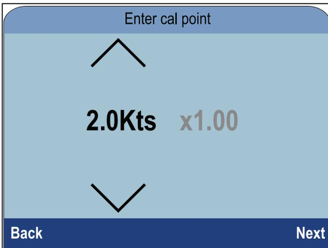
3. Use the **Up** and **Down** buttons to select the desired speed that you want to add a Calibration Point for.
