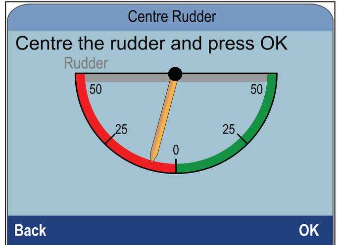
8. Turn the steering until the Rudder is centred.
