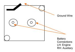
CAUTION: Connect battery connections first. Then connect ground to a common negative point or either battery negative.
