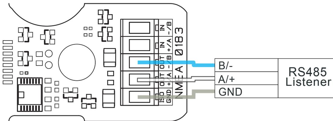
Figure 5 – RS485 / IEC 61162-2 port connections
