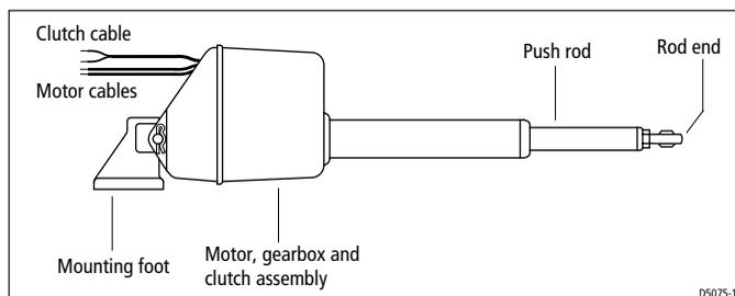
Figure 1: Main parts of the linear drive
