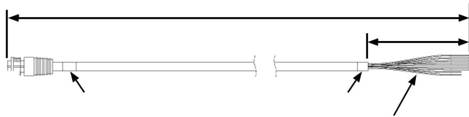
The receiver end of the cable is terminated with an environmentally sealed 12-pin connection while the opposite end is unterminated and requires field stripping and tinning.
