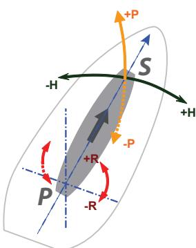
Mount the HS70 parallel to, and along the centerline of, the axis of the boat. This provides a true heading. In this orientation:
