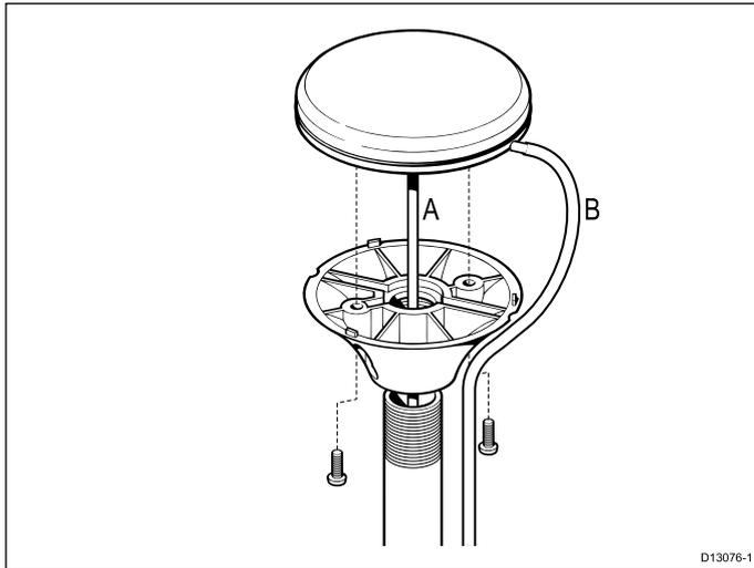
1. Ensuring that the *Antenna location requirements* are met, securely attach the pole to a suitable, stable point.
