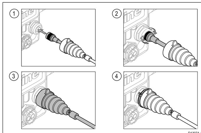
1. Fully insert the antenna's cable connector into the GA150 connector on the rear of your display.
