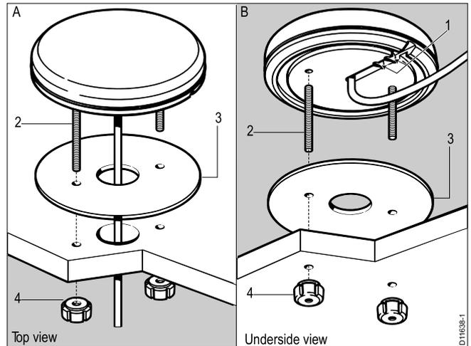
2. Screw the two mounting studs (2) into the underside of the antenna.
