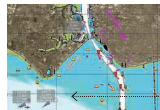
Radar Overlay Overlay AIS targets radar contacts on Raymarine multifunction navigation displays.
